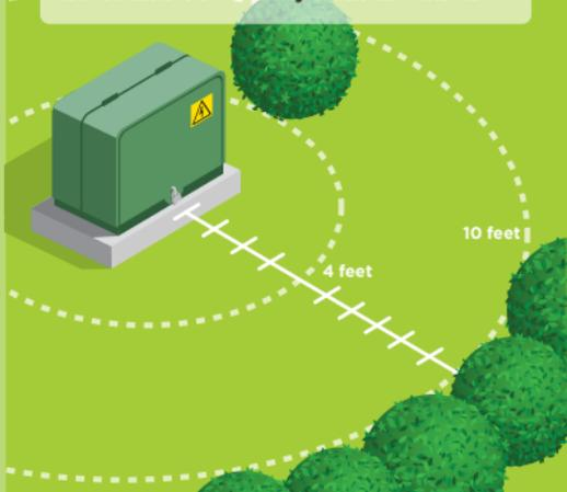
Never dig near a pad-mounted transformer. They are surrounded by underground cables. Hitting the cable could result in electrical shock or disruption of service.
